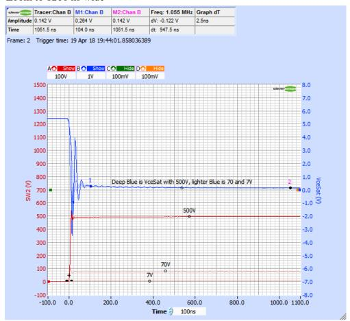
Chan A is the opposing switch - SW2. Chan B is the CS1110 V<sub>CE Sat</sub> probe output.
