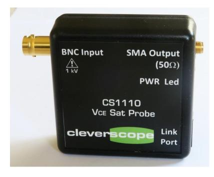
The BNC input is connected via coax to the UUT. Do not use a scope probe as it has >300 ohm series resistance which will deliver incorrect results.
