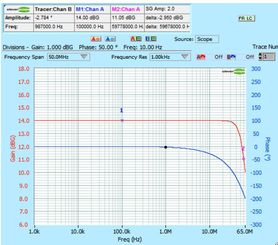
Gain is 14 dB (x5 with 50 ohm termination).
