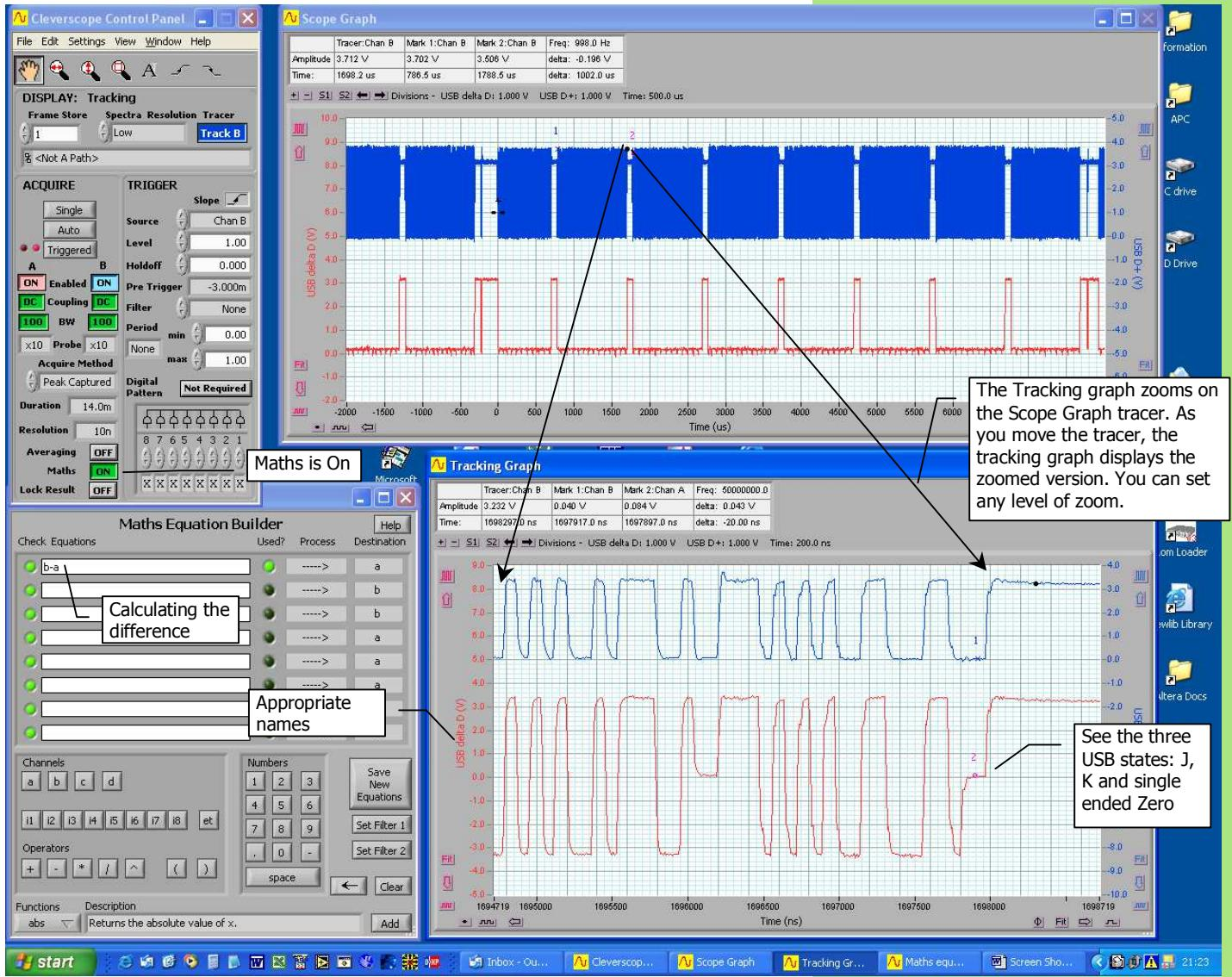
The Maths Equation Builder can be used to build equations of considerable complexity. All the standard mathematical functions (abs, log, power, trig functions, thresholding functions), and standard operators + - \* / ^ ( ) are supported. In addition Process supports integration, differentiation and filtering. You can store intermediate results in any channel (a-d, i1-i8), and use them in the next equation.
