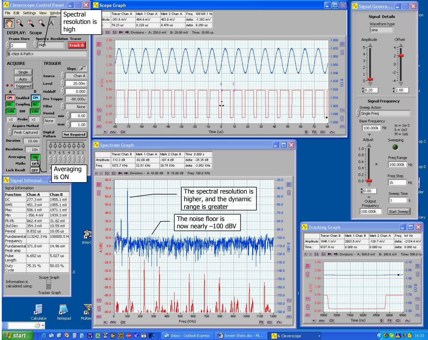
We can set the transform type (RMS Amplitude, Power, Power Density, Gain/Phase) and the FFT Window used (Hanning, Hamming, Blackman-Harris, Exact Blackman, Blackman, Flat-top, Low sidelobe) to suit the type of signals we are investigating.
